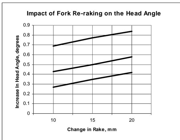
In this plot, the three lines represent different levels of reduction in the fork length (FL), as a consequence of the re-raking process.
