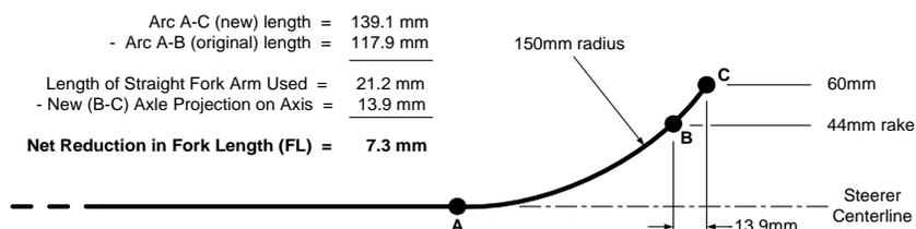
Two conclusions are clear. First, the inescapable reduction in fork length (FL) as the result of this manipulation will combine with the effect of the increased rake to further reduce the fork's length-on-axis (FLA). As a result of the steeper head angle, less rake than initially figured will be adequate to provide the target value for trail. And second, the process of re-raking a fork can be done well, or it can be done poorly when it comes to preserving tire clearance and brake reach.
